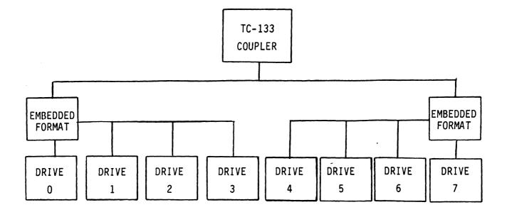
FIGURE 2.4 Example Tape Formats
