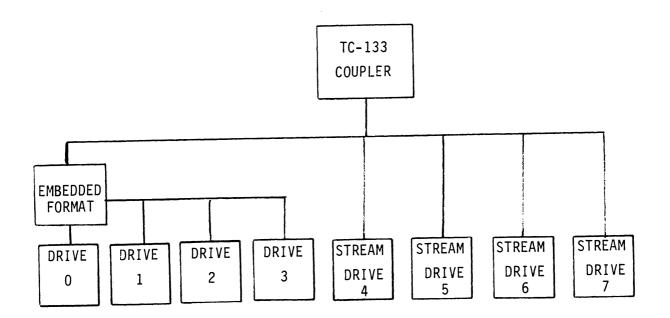
FIGURE 2.3 Daisy-Chaining - Two Embedded Formatters
